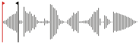
Fade In applied at the start of the audio to create a smooth volume transition to begin.
